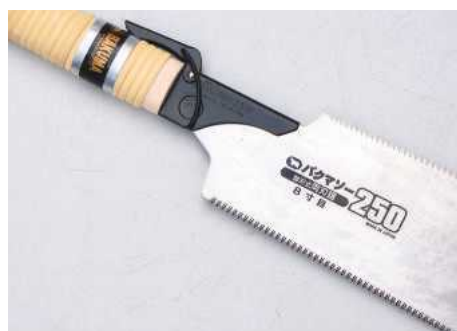
▲ One edge on the Bakuma Ryoba saw has finer teeth, whereas the other has bigger teeth
